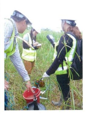
Surface water sampling and onsite measurement at SW-3
