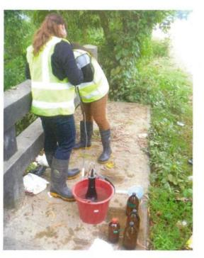
Surface water sampling and onsite measurement at SW-2
