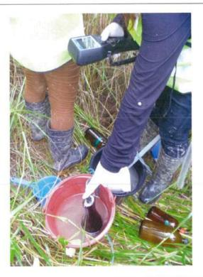
Surface water sampling and onsite measurement at SW-4
