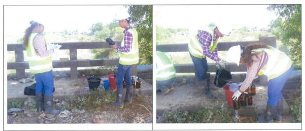
Surface water sampling and onsite measurement at SW-2
